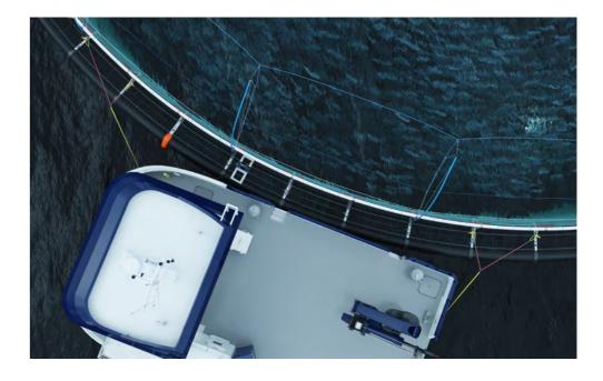
Large Boat Mooring ensures safe and gentle mooring of wellboats and larger vessels while extending the lifespan of the floating collar and reducing stress on the mooring brackets. With easy installation and efficient load distribution, this solution enhances operational reliability and minimizes unexpected maintenance needs.
