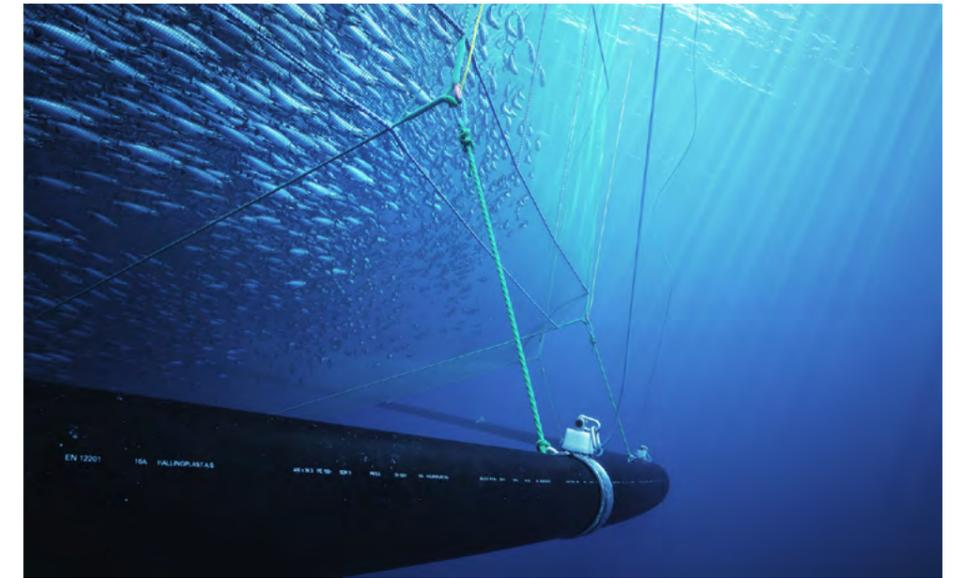
A sinker tube helps prevent the shape and thus the net volume from changing in locations subject to many storms. The sinker tube is designed to make the handling of the net easier.
