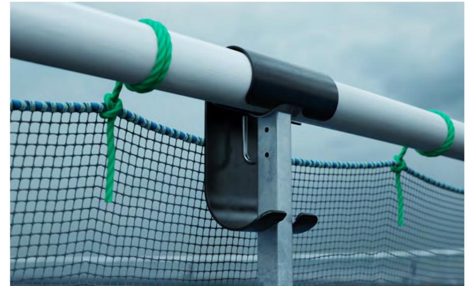
The ScaleAQ net hook protector/HSE fitting prevents nets and ropes from catching on net hooks on the inside of the handrail when the net is pulled over the edge. The net hook protector also prevents crushing injuries.
