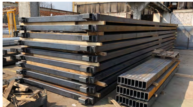
Steel pen sections before galvanization
