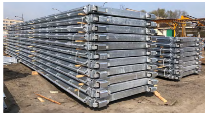
Steel pen sections after galvanization
